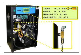
When the Compressor runs for 3:00 minutes (unless adjusted to a different Set Point by the user), a High Compressor Last Run Time (LAST RUN) alarm should appear on the System Screen.
