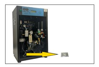
**6.5.5** Remove and discard the packing foam blocks from around the Compressor.
