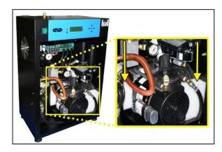
**6.5.6** Remove the Plug from the Outlet Port by pressing the ferrule down then pulling the plug upward.
